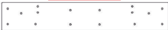
C01 GUIA SUPERIOR DE LA VIGA DEL COLUMPIO - W4L18968 (x1) 1 3/8"x6 3/4"x40" (36x172x1017)
