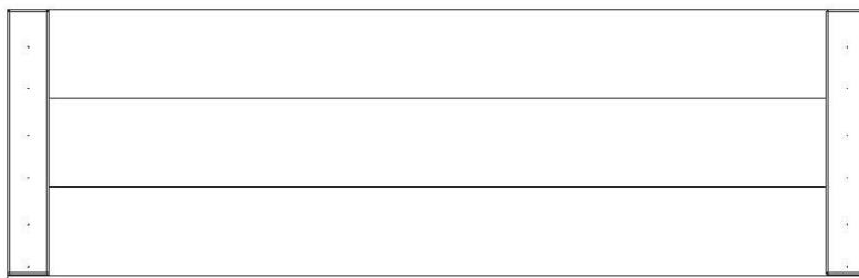
RP2 PANEL DE TECHO SUPERIOR - W2A03795 (x3) 1 5/8"x15 5/8"x59 3/8" (42x396x1241)
