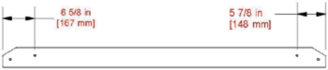
AD02 GUIA DE PARED - W4L18979 (x2) 1"x3 7/8"x65 3/4" (24x100x1670)
