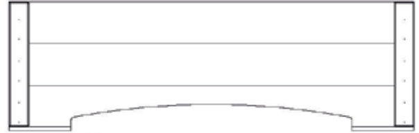
RP3 PANEL DE TECHO - W2A03796 (x1) 1 5/8"x15 5/8"x59 3/8" (42x396x1241)
